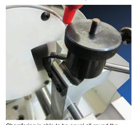
Chamfering is able to be equal all-round the stem end by the chamfering end stop system.
