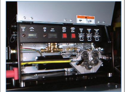
**Wire counter** Re-settable LCD meter that displays wire fed in feet/meters during spray operation.
