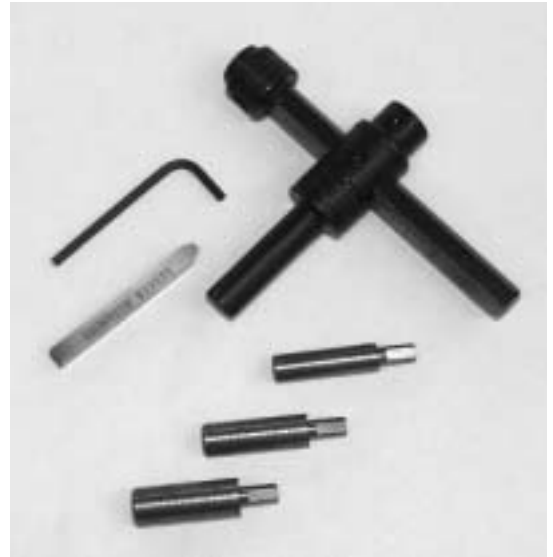
Complete Cylinder Head Grooving Tool-Cummins
