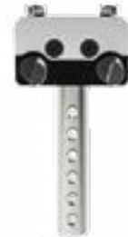
Dual pin trip design eliminates starwheel timing
