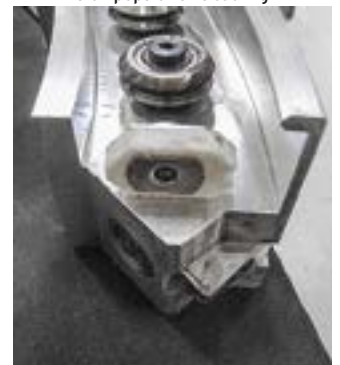
V-Lock ring mating surface resists force distortion
