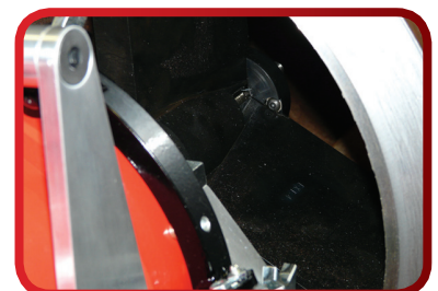
Wachs EP424 machines complex weld prep profiles with a precision lathe type finish and no heat affected zone.
