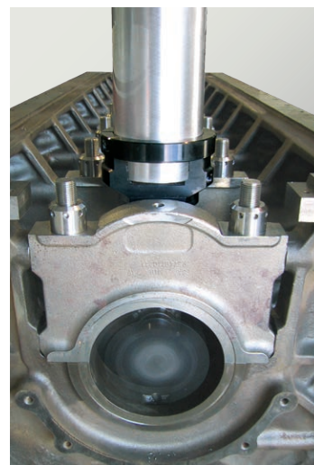
Special steel main bearing housings found in high power diesel engines such as MTU 4000 require high speed machining to obtain superior accuracy of roundness, straightness, parallelism and surface finish.
