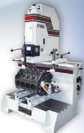
F10A Programmable CNC Cylinder Boring and Resleeving Machine
