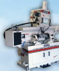
SG10A CNC Cylinder Head Seat & Guide Machine
