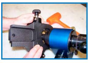
Select jaw set according to the ID diameter that the machine will chuck into.
