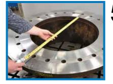
Set machine onto flange using setup fingers. Lightly tighten leveling feet in the flange.
