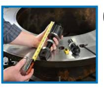
Extend feet into flange. Indicate, level and tighten leveling feet and stationary feet.
