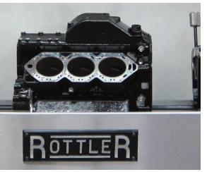
Marine Outboard, Snowmobile, Motorcycle and other similar cylinders can be easily mounted and rolled over for precision blind hole honing.
