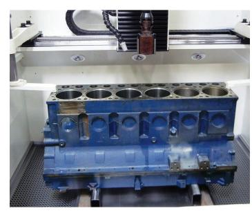
**Universal Quick Clamp Handles** Universal Quick Clamp Handles allow for rigid clamping of small single cylinders. Large Inline diesel blocks utilize the Quick Clamp System for fast and versatile set up.
