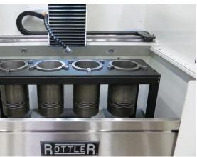
Special Liner Honing Fixture allows multiple liners to be clamped and honed with the same setup. The Multiple Liner Honing Fixture is shown here with four CAT 3500 liners. Fixtures for smaller cylinders such as Harley can hold up to six or eight liners/cylinders. Profit from the lucrative business
