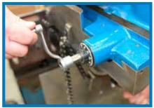
Rapid longitudinal travel can be made with a drill motor for quick set-up.
