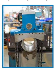
The 2.0 inch (50.8 mm) lateral travel of the KM4000 allows you to cut wide keyways or slots with a less expensive, smaller end mill. The calibrated cross slide is positioned with the hand crank.
