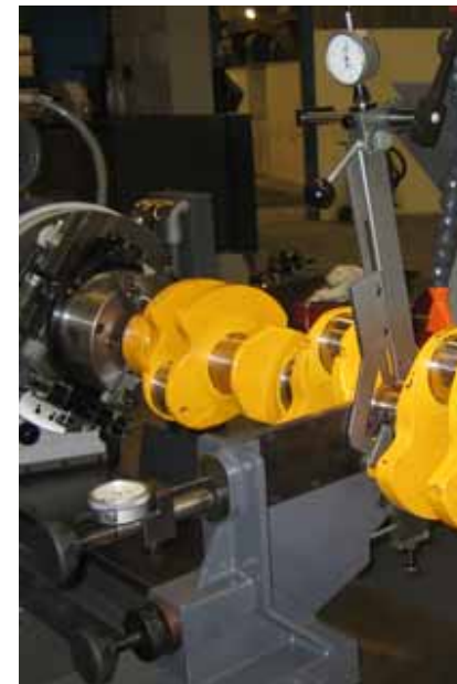
Continuous journal sizing gauge AZ 770 (recommended equipment) and hydraulic steady rest (optional equipment)
