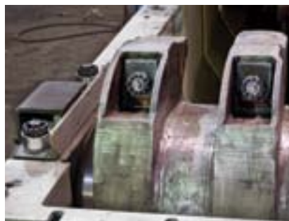
The bolting challenges on this crusher included limited space and extreme working conditions. Multi-jackbolt tensioners proved to be the ideal solution. Only 43 lb•ft (58 Nm) of torque on the jackbolts was needed, the equivalent torque on the standard bolt is 2,150 lb•ft (2915 Nm). The use of a small 3/8" drive hand held torque wrench was much safer and more accurate than previous bolting methods.
