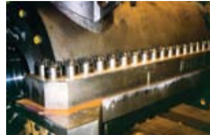
Fiftytwo 2" (50,8 mm) tensioners on this centrifugal compressor were tightened by two men in 2-1/2 hours. The old method required three men working an eight hour shift.
