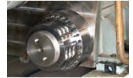
Split-Nut thrust collars are a custom designed product from Superbolt that are much easier to install and remove than other large threaded fasteners on large press columns.
