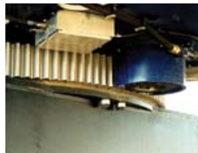
Large power shovels have many critical bolting applications. Multi-jackbolt tensioners are used extensively on these machines, all over the world. Seen above, MT tensioners on a ring gear.
