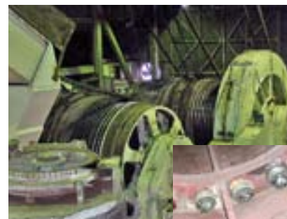
On these hoist & drag drums, the high preload of 428,400 lbf (1906 kN) was achieved with only 233 lb•ft (316 Nm) of torque required on each jackbolt. The added flex from the Superbolt tensioners more than doubled the elasticity of the bolted connection.
