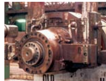
Thrust collars on bearing chocks create higher preloads than the previous method and therefore even the heaviest peakloads can be absorbed. The roll necks are lasting and the production runs smoothly.
