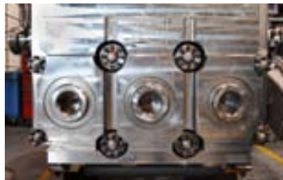
With a 2,500 horsepower rating, and 273,000 lb (1215 kN) rod load, this Weir SPM Destiny™ Fracturing Pump utilizes Superbolt tensioners to make bolting safer and easier in the field, as only hand tools are needed.
