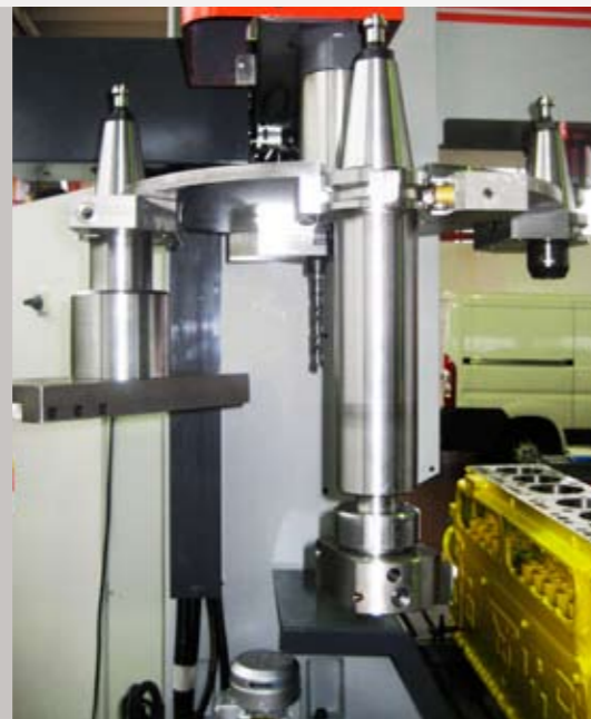
Automatic Centering and Tools Changing
