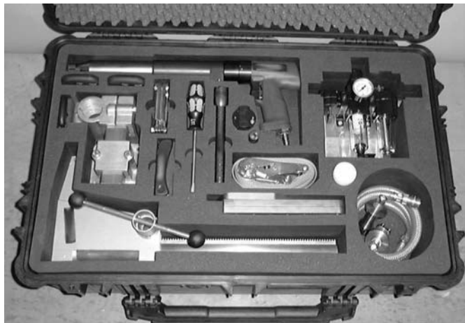
VM2150 with pneumatic motor (standard scope of supply does not include maintenance unit)
