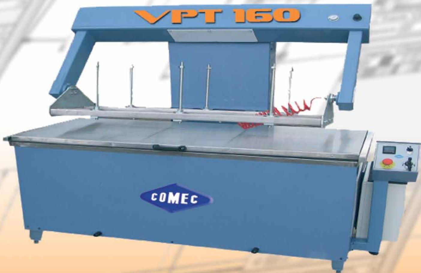
**VASCA PER PROVA TENUTA DI TESTATE E MONOBLOCCHI**
